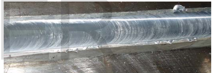
Fig. 2 Picture of as-processed plate with one pass at 500 rpm, 20
